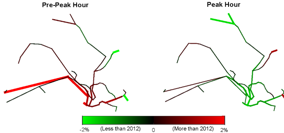
Fig 5. Change to passenger flows from Sept. 2012 to 2014, down direction (Halvorsen et. al., 2016)
