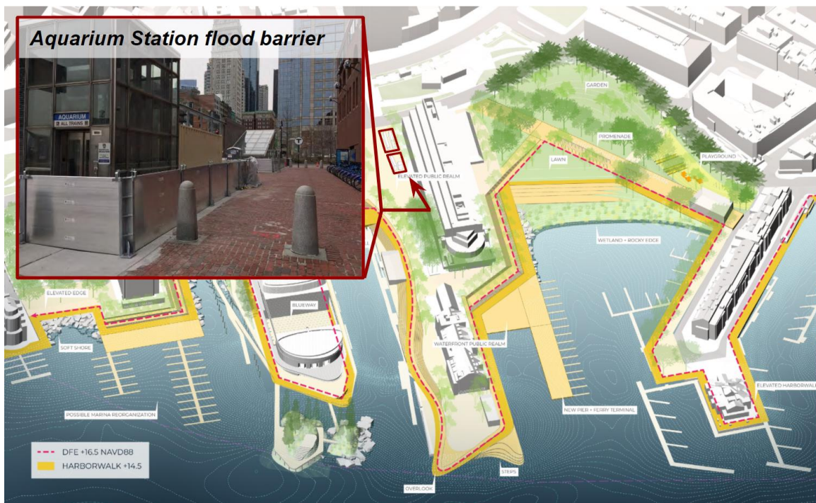
Figure 5: Example of neighborhood-level adaptation plan proposed for Long Wharf in Downtown Boston (City of Boston, 2020b). Inset: example asset-level adaptation project (deployable flood barriers) recently completed to protect entrances to the MBTA Aquarium Station (MassDOT, 2021b).
